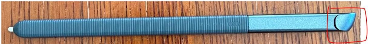
Opposite side of stylus, which should face into the tablet.
